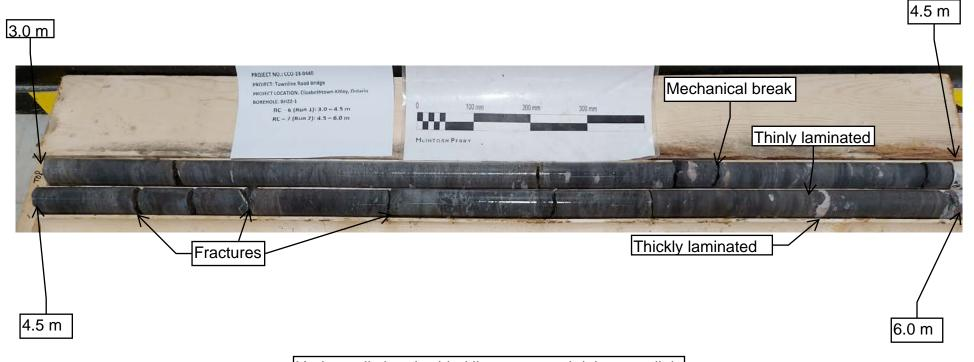
Horizontally interbedded limestone and dolostone, light to dark grey, laminated, slightly to moderately fracture. Possible mineral composition: Calcite, and dolomite.
