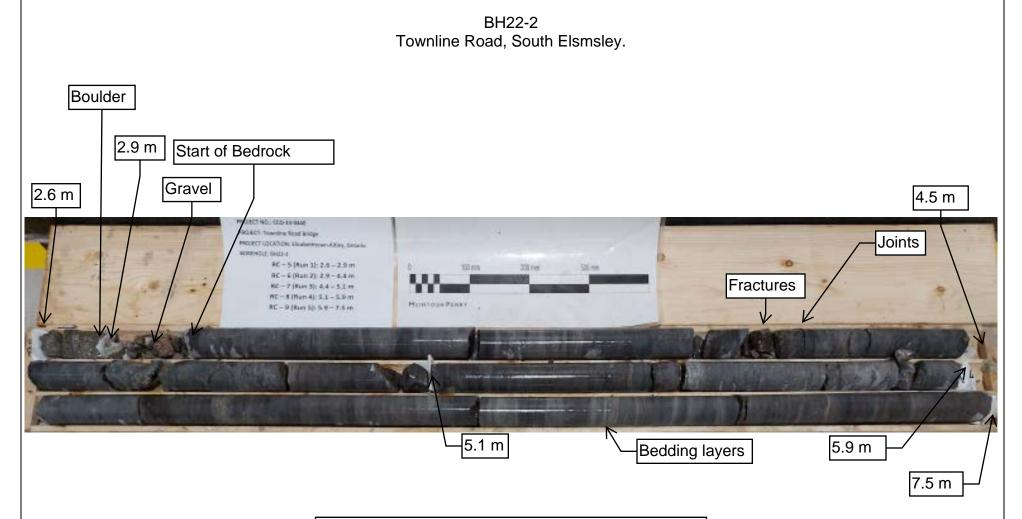
Horizontally interbedded limestone and dolostone, light to dark grey, laminated, slightly to moderately fracture. Possible mineral composition: Calcite, and dolomite.
