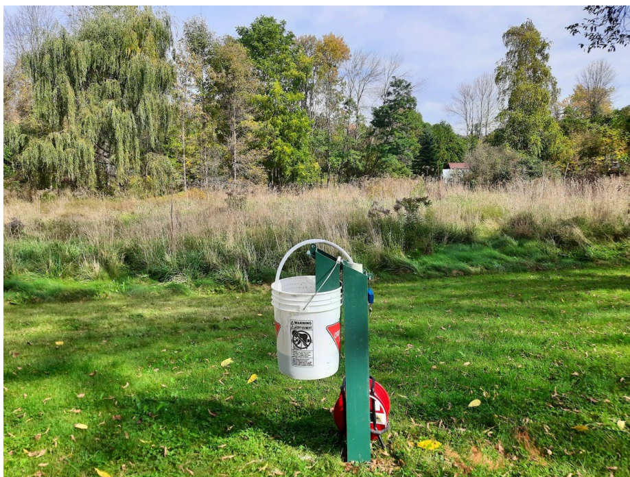
Photo 2 BH101 completed with a monitoring well, October 2023.
