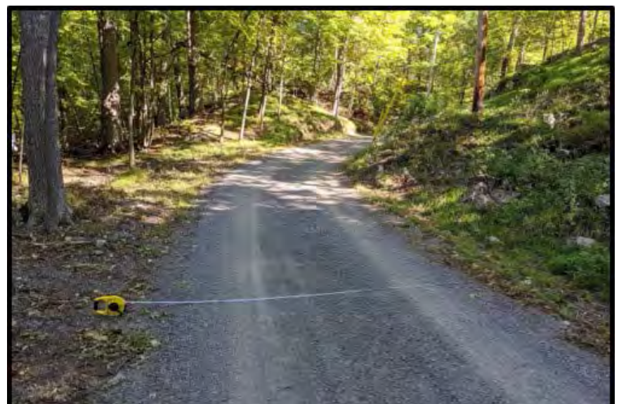
Photo 7: Shows how the width of roads were found, a spike was put into either side of the road and the measurement was taken from the edge of the opposing side. About halfway through a measurement wheel was used, to save time and speed up the process.
